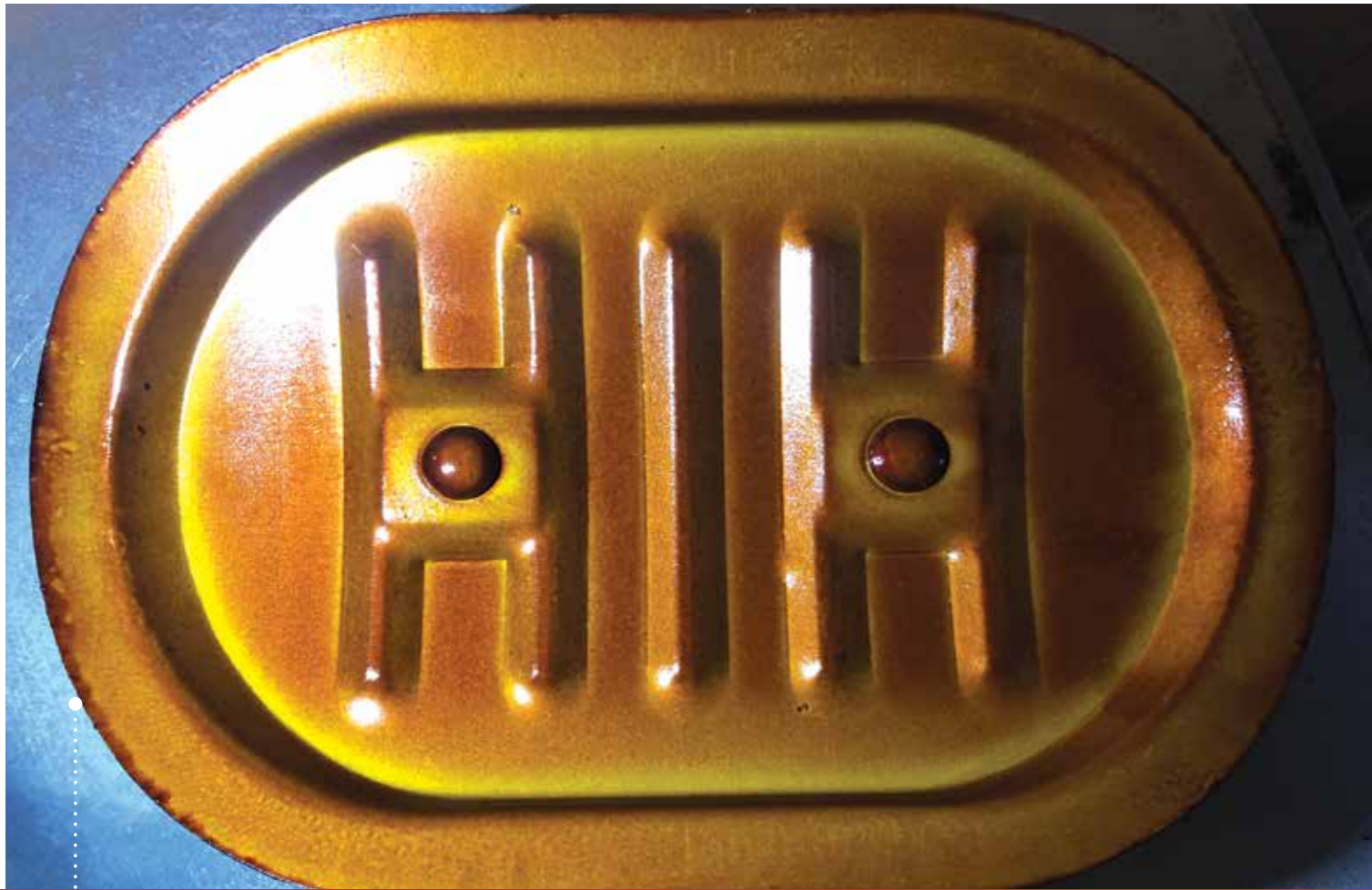
Inspection Hatch with JIMCO Technology - Not cleaned for 60 months
